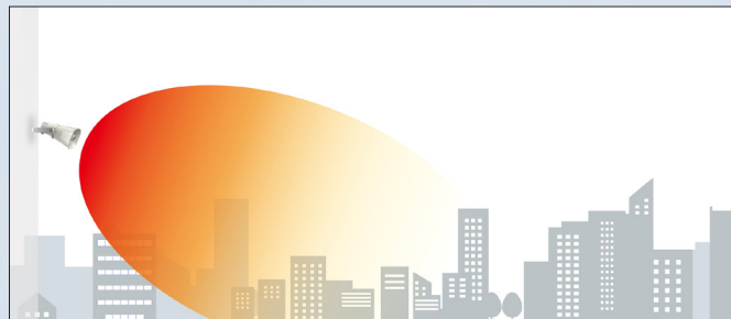
Sound Dispersion of the Conventional Horn Speaker
