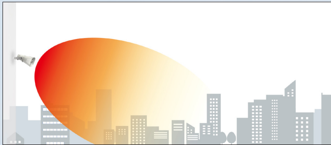
Sound Dispersion of the Conventional Horn Speaker
