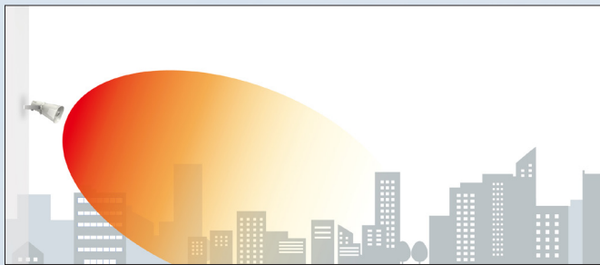
Sound Dispersion of the Conventional Horn Speaker
